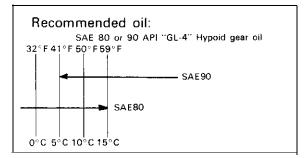
If desired, an SAE 80W/90 hypoid gear oil may be used for all conditions.
