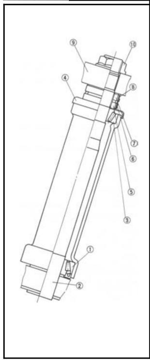
@Checkthe steering stem by turning it lock to lock. If there is any binding, remove the steering stem assembly and inspect the steering bearings ① ③
