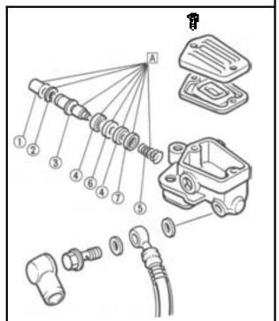
Front Brake Master Cylinder Disassembly
