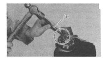
2. Lock the threads with center punch ① as shown.
