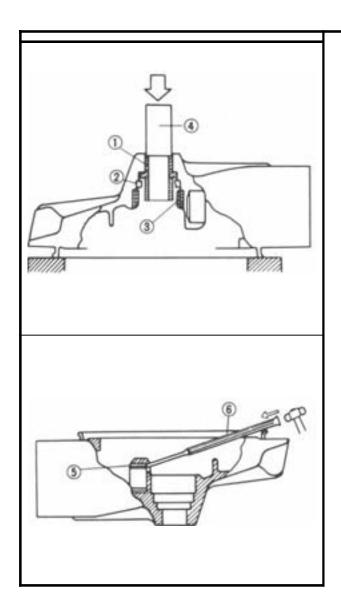
Bearing Removal and Reassembly
