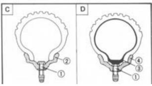
Be sure to install the correct tube when using tube type tires.
