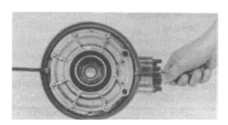
Ring Gear Stopper Clearance Measurement
