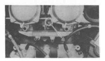
Carburetor synchronization adjustment steps: .Synchronize carburetor No. 1 to carburetor No. 2 by turning synchronizing screw "A" until both gauges read the same.
