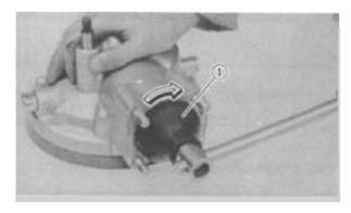
Final Drive Gear Disassembly
