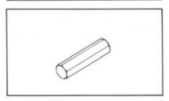
Front Fork Cap Socket (17 mm) P/N YM-01104
