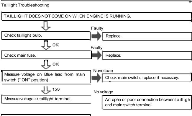
Poor ground or poor connection of taillight wiring.
