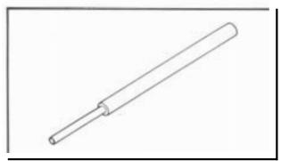
4. Valve Guide Remover (5.5 mm) P/N YM-01122
