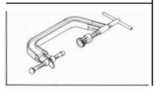
3. Valve Spring Compressor P/N YM-04019
