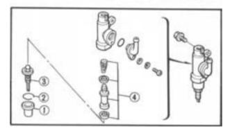
Rear Brake Master Cylinder Disassembly
