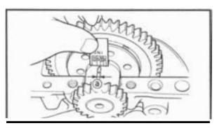
• Tighter the bolts to specification in the tightening sequence cast on the crankcase.
